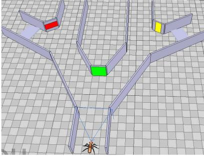
Fig. 2. Simulation set-up developed in the V-REP dynamic environment. A fly-inspired legged robot is asked to walk in a multiple Y-maze environment selecting the suitable route and motor actions through the processing of visual cues acquired from landmarks placed in each selection chamber.
