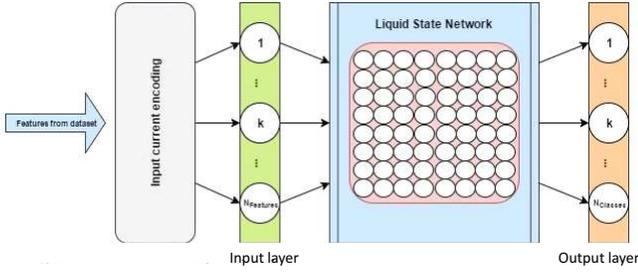
Fig. 1. Block scheme of the MB-inspired developed architecture devoted to classification. The external input is pre-processed by a layer that randomly excite the lattice of locally connected spiking neurons. The spiking activity is exploited for classification using multiple read-out maps in the output layer that are trained to distinguish the different presented classes.
