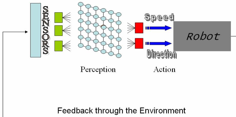
Fig.10: Scheme of the perceptual framework used for navigation control. The framework is divided into functional blocks, starting from the sensing layer to the robot motor control stage. The RD CNN extracts the needed information from sensors creating an internal representation through Turing Patterns generated. The learning process is guided by a motivation assigned to the robot.
