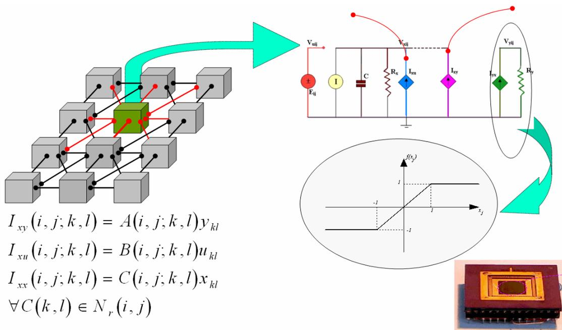
Fig.2 The Cellular Nonlinear Network scheme and main characteristics
