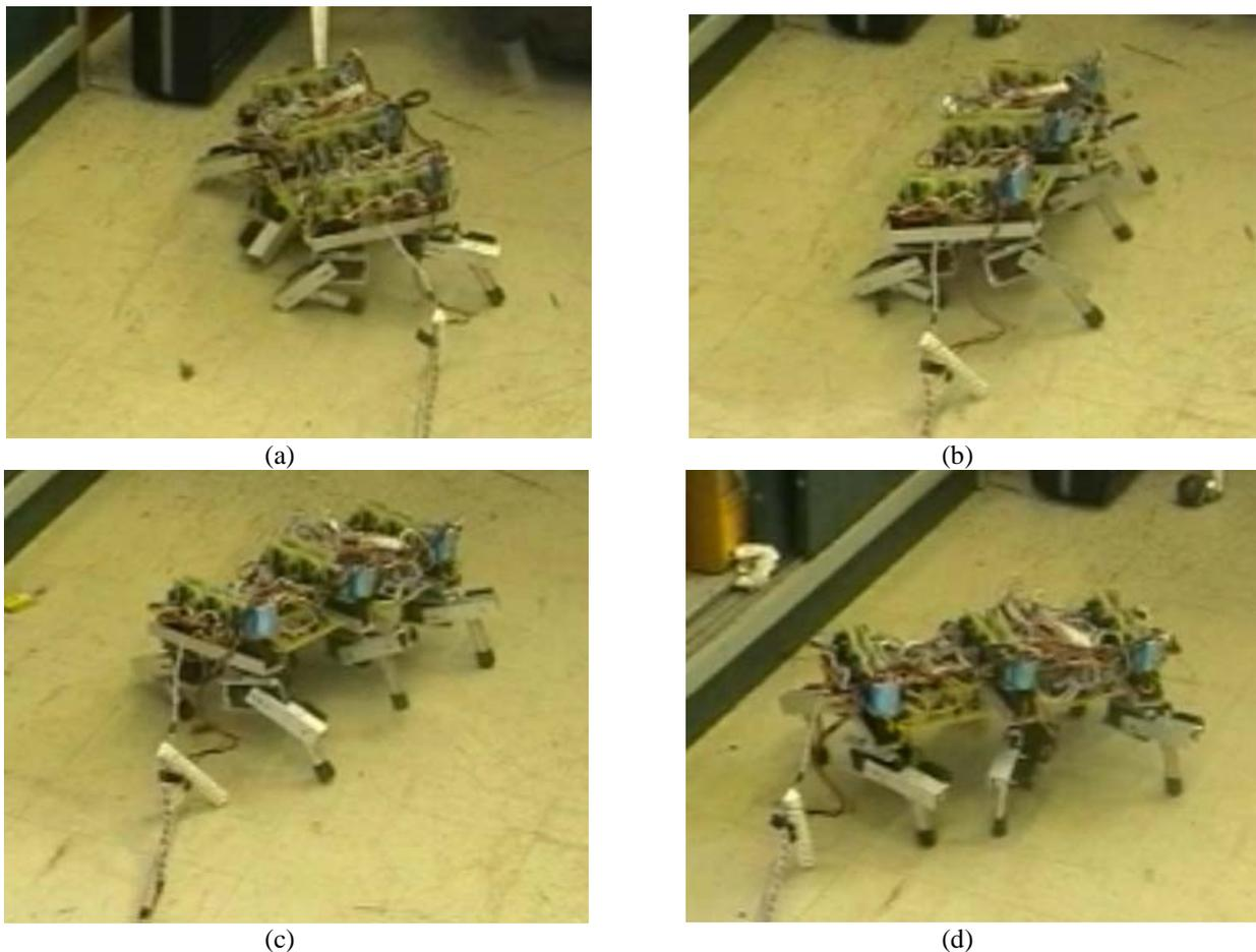
Fig.9: (a) Rexabot III front right leg is overloaded; (b)-(c)-(d) emergence of a recovery strategy coming from the integration among the CNN locomotion controller and the analog attitude controller.
